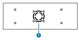
**1** Fan Ventilator: These are air ventilation areas, DO NOT block these areas or cover it with any object. Please allow adequate space around the unit for air circulation.
