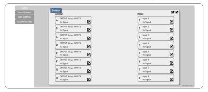
Click on 'Data Routing' page to set up Output Baud rate and Uart Routing status.
