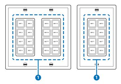
1 Macro Buttons: Each button contains 2 color LEDs (red and blue) with adjustable individual brightness levels from 0~100. Each button can activate a customized macro. (For further detail on these settings please refer to section 6.5 "WebGUI Control".)
