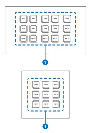
1 Macro Buttons: Each button contains 2 color LEDs (red and blue) with adjustable individual brightness levels from 0~100. Each button can activate a customized macro. (For further detail on these settings please refer to section 6.5 "WebGUI Control".)
