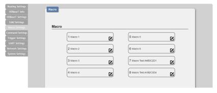
Click on the "Macro Settings" tab to execute/edit the 8 available macros. These macros can be executed by activating the 8 input triggers on the back of the unit as well as via the WebGUI or Telnet. Each macro can contain up to 16 individual commands.
