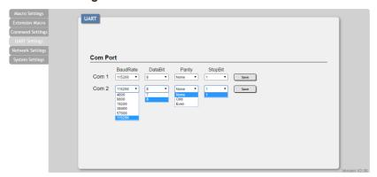
Click on the "UART Settings" tab to configure each COM port's Baud Rate, Data Bit, Parity, and Stop Bit. Values that can't be directly selected here may be set via Telnet or RS-232. After changing a COM port's settings please click on the "Save" button to store the new settings.
