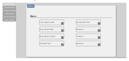
Click on the "Macro Settings" tab to execute/edit the 8 primary macros. These macros can be executed by activating the 8 input triggers on the back of the unit as well as via WebGUI, Telnet, or IR remote. Each macro can contain up to 16 individual commands.
