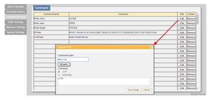
Click on the "Command Settings" tab to create, edit or delete commands. The number of commands that can be stored in the unit is limited by memory. It is generally recommended that commands be under 128 characters long (including spaces). However, if longer commands are needed there is limited support for commands up to 512 characters long. In this case the number of (up to) 512 character commands is limited to 32 and the remaining 96 commands must be under 128 characters.
