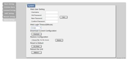
Click on the "System Settings" tab to make changes to various system settings. From this tab you can change the WebGUI login password and login timeout settings. You may also save the full system configuration, including all macros, to your connected PC/Laptop or restore them from a previously saved configuration. Finally, this tab provides buttons to reset the unit to factory defaults and to reboot the unit.
