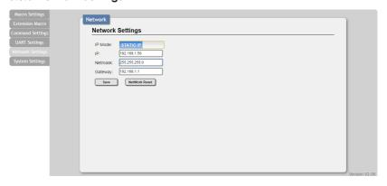
Click on the "Network Settings" tab to change the network settings for the unit. You can manually set the IP address, netmask, and gateway address in "Static IP" mode, or you can obtain an IP address automatically by enabling DHCP.
