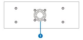
1 Fan Ventilator: These are air ventilation areas, DO NOT block these areas or cover it with any object. Please allow adequate space around the unit for air circulation.
