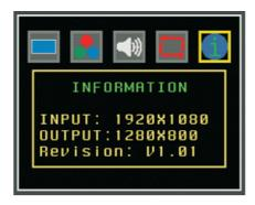
• Displays the source input format, the output display format and the unit's software version.
