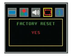
Selects YES to return the unit to the factory settings. The default Factory Setting for Video display is 'Full Screen' (1024×768@60Hz), Color setting's factory default rate is the same as shown on the OSD and SDI audio is 'AUTO'.
