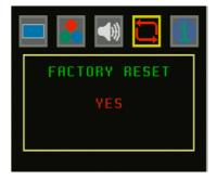
Select YES to return the unit to the factory settings. The default Factory Setting for Video display is 'Full Screen' (1280×720@60Hz), Color setting's factory default rate is the same as shown on the OSD and SDI audio is 'AUTO'.
