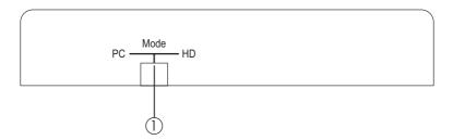
PC/HD switch: This slide switch allows you to select PC or component HD timing output. Simply slide the dip switch to left or right and the output mode will display your desire selection.
