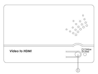
CV/SV SW & LED: Press this button to switch input source between composite or S-Video. The Led will illuminate in yellow when switch to composite input and red when switch to S-Video input.
