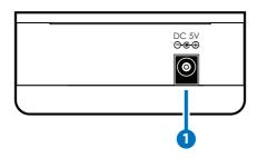
**1 DC 5V:** Connect the 5V DC power supply to the unit and plug the adaptor into an AC wall outlet.
