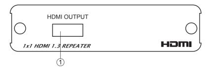
1 HDMI Output: Connect output port to the HDMI display.
