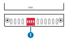
1 EDID: The EDID dipswitch block provides a way to select the EDID to use with the connected source. By using a combination of on and off settings for the dipswitches, there are a total of 16 possible EDID selections across 3 different operation modes.
