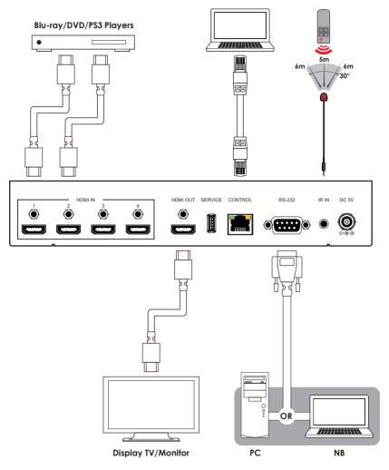
**Note:** The IR Extender cable distance is up to 5 meters and 8 meters for the IR Window on the front panel.
