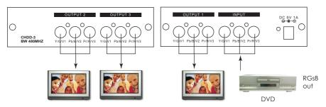
3. Works as a three 1-in 3-out distribution amplifier for composite video source.
