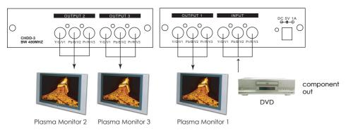
2. Works as a 1-in 3-out distribution amplifier for HD RGsB (Sync on Green) video source.
