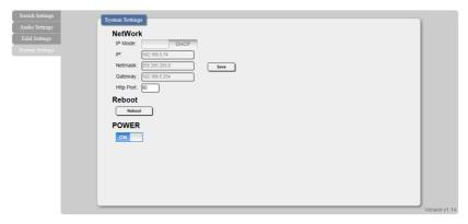
Select IP Mode with STATIC IP or DHCP for using a static or floating IP.
