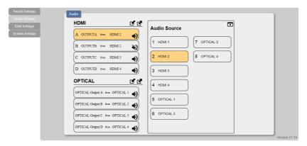
Click on HDMI/Optical output(s)  $A\sim D$  to select an Audio Source from  $1\sim 8$ , multiple output may be selected for an input setting. To save the setting click on  $\blacksquare$  and to recall the setting click on  $\blacksquare$ . To mute and unmute the output audio click on  $\blacksquare$ .
