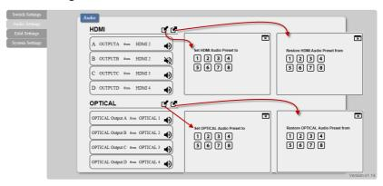
You may rename outputs and inputs devices by click on **2** to bring out the rename window. Type in the new name under Set OUTPUT/INPUT Name and click on **1** to save it. Inputs HDCP setting can be selected under this window.
