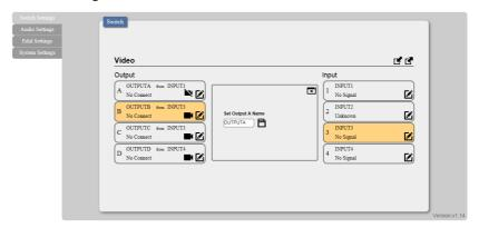
Click on OUTPUT A~D to select output display with INPUT 1~4 source selection, multi-outputs can select an input or an output with an input selection. Once the selection is made on both output and input successfully, the background color will return back to white.
