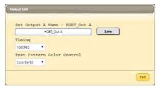
2) Output Edit: Clicking on the "Edit" icon (\*) for an output provides a way to change the name of the output. It also provides control over the test pattern resolution and style used when the "Pattern"
