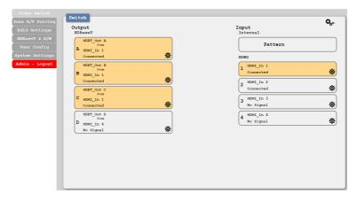
1) Output and Input Routing: To begin assigning a new video route, please click the button of the HDBaseT output you wish to send video to and then click on the button of the preferred HDMI input port or Pattern. If desired, you may select more than one output prior to selecting the input. As you select each button they will change their color to orange. The new route will become active immediately and the routing information displayed on the buttons will change accordingly.
