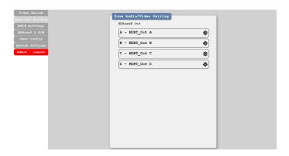
After configuring the button pairing for a zone, the user can change the routing in whichever zone they are currently located simply by pressing a number key on the remote control. The discrete zone pairings can also be activated from within the WebGUI or by using Telnet/RS-232 commands.
