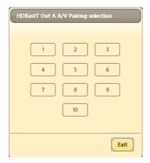
2) Quick Button Selection: To activate an audio/video pairing from the WebGUI, select the preferred output zone (A~D) to launch its selection window. The numbers 1~10 correspond to the keys on the remote control and hovering the mouse over each button will reveal the routing currently associated with it.
