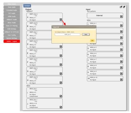
All inputs and outputs can be renamed as required. To rename the HDBaseT output ports and HDMI input ports please click the "edit" icon (2). Click the "Save" button to confirm the change.
