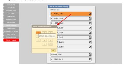
Please select the HDBaseT output port first and then click the "edit" icon (🗹) to launch the window for further adjustments. The numbers 1~10 and "pattern" correspond to the keys on remote control unit.
