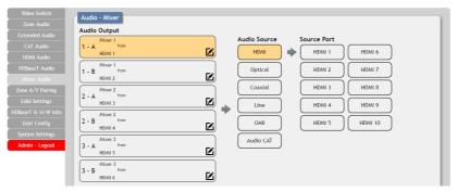
Click the buttons from left to right to choose each mixer's A & B sources. Only 2 sources total may be selected for each mixer. Once the new source has been selected, the change will happen immediately. Audio source options include HDMI, Optical, Coaxial, Line. OAR and Audio CAT.
