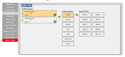
Click the buttons from left to right to choose each output's source. Once the new source has been selected, the change will happen immediately. Audio source options include HDMI, Optical, Coaxial, Line, OAR, Audio CAT and Mixer.
