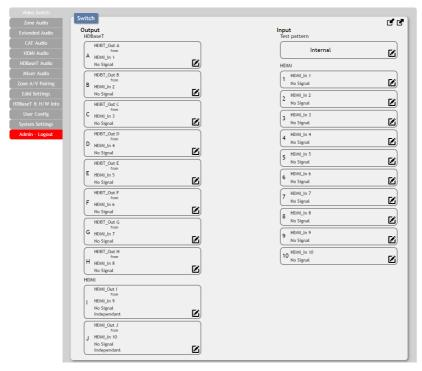
To begin assigning a new video route, please click the button of the HDBaseT output you wish to send video to (e.g. "HDBT\_Out A") and then click on the button of the preferred HDMI input port (e.g. "HDMI\_In 1"). If desired, you may select more than one output prior to selecting the input. As you select each button they will change their color to orange. The new route will become active immediately and the routing information displayed on the buttons will change accordingly.
