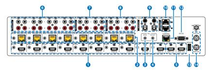
1 HDMI IN & IR OUT 1~10: Connect up to 10 source devices to the HDMI ports using appropriate quality HDMI cables. Input source devices include Blu-ray players, set-top boxes, game systems and so on. These inputs are DVI-D compliant (with the use of DVI to HDMI adapters or cables). Attach IR blasters to the IR Out ports to transmit the IR signals received from connected HDBaseT Receivers. The IR signal routing follows the HDMI signal routing.
