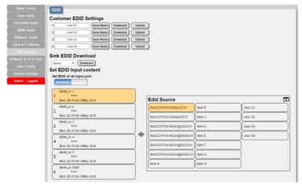
The Set EDID Input Content section allows for the assignment of an EDID to each individual input port, or to all inputs at once. Click the selection bar to toggle between individual assignment, or all inputs.
