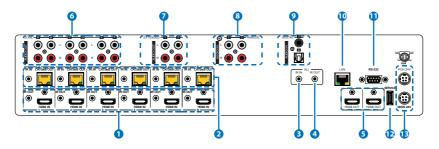
HDMI IN & IR OUT 1~6: Connect up to 6 source devices to the HDMI ports using appropriate quality HDMI cables. Input source devices include Blu-ray players, set-top boxes, game systems and so on. These inputs are DVI-D compliant (with the use of DVI to HDMI adapters or cables). Attach IR blasters to the IR Out ports to transmit the IR signals received from connected HDBaseT Receivers. The IR signal routing follows the HDMI signal routing.
