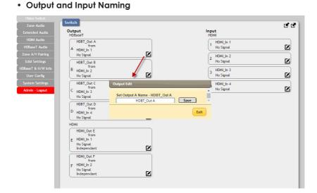
All inputs and outputs can be renamed as required. To rename the HDBaseT output ports and HDMI input ports please click the "edit" icon (**S**). Click the "Save" button to confirm the change. Note: Blank spaces ("") are not allowed in names.
