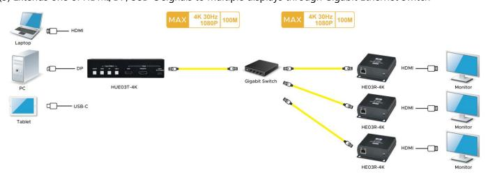
\* EEE(Energy-Efficient Ethernet) function must be turned off, when connect to Gigabit Ethernet Switch.
