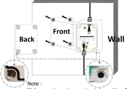
Make sure to put correct notch position for the upper case.
