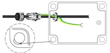
Note : The position of grounding cable must be same as left diagram.
