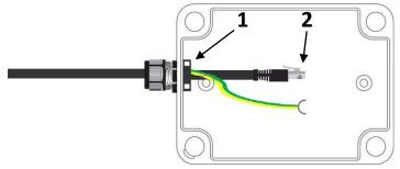
6. The other end is also connected to the RJ45 connector, and make the nut locked into (1)(2) the waterproof set.
