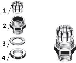
3. The pre-assembled network and grounding cables to pass through the waterproof cover set as shown.
