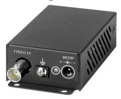
The GL001HD Video Ground Loop Isolator is an active devices which reduce ground loop interference without any video loss on HD CCTV signals. It could be easily install in a new or added to existing systems. It is useful where a video signal is transmitted via cable between points with different ground potentials, differences in ground potentials are typically caused by unbalanced power line loads.
