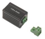
The RS003 USB Converter provides an easy solution for adding new or additional Com Ports to Windows or Macintosh computers through their USB ports. The RS485 connection is 2- pin terminal connector. The unit is powered from the USB connection, so no external power supply is necessary.
