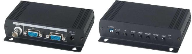
This VGA to BNC converter also features a VGA output port that allows for VGA Loop-Through. You can simultaneously view video on a VGA monitor while viewing the video on your CRT ,TV monitor. It convert your VGA signal to be viewed on any TV, projector, or any other viewing device that uses standard BNC (RCA) connector with this simple external device.
