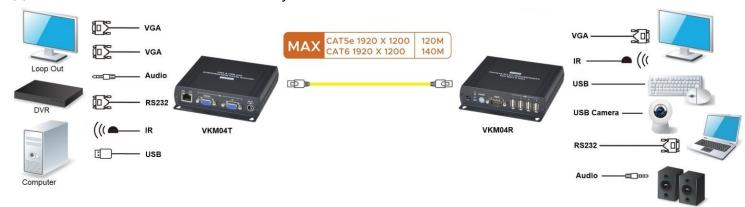
(2) Works with optional model SR01 for extra 140M over CAT6 cable, 120M over CAT5e cable.
