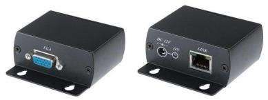
VE01H is designed to extend high resolution 1920 x 1200 VGA signal with audio over cost effective CAT5e/CAT6 cable up to 70M. There is no external power requested at receiver unit for easy installation at monitor side. The idea application could be to move multimedia content from player to display and could be used in shopping malls, public address systems, airports, train & bus station, boardrooms, trade shows, computer based training application.
