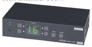
HDMI Extender Over Coax extends an HDMI signal over a point-to-point coax cable up to 500M with RG59/RG6 coaxial cabling. The HDMI Extender Over Coax allows the capability to split to multiple receivers, or combine multiple transmitters set to different channels, using simple CATV splitters or combiners. It could be widely applied in CCTV, CATV, outer large screen, shopping mall advertisement, media education or replace new HDMI devices instead of old analog system over existing coaxial cable.
