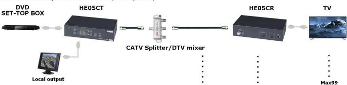
Multiple TX to multiple RX connection (with splitter)
