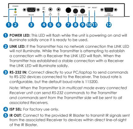
6 IR IN: Connect to the provided IR Extender to extend the IR control range of remotely located devices. Ensure that the remote being used is within direct line-of-sight of the IR Extender.
