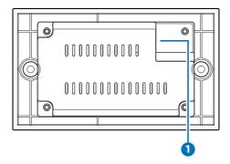
1 CAT5e/6/7 IN: Connect to the transmitter unit with a single CAT5e/6/7 cable for transmission of all data signals.
