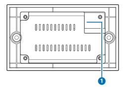
**CAT5e/6/7 IN:** Connect to the transmitter unit with a single CAT5e/6/7 cable for transmission of all data signals.
