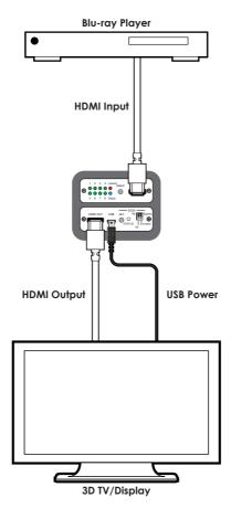
Note: In this example the unit is powered by a USB port on the TV/Display. It can also be powered by a compatible device that can provide power over HDMI.
