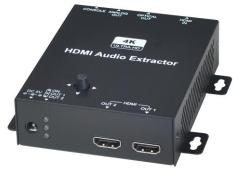
The HAE01 is an HDMI multifunction tool: allow you to extract 4K HDMI for both digital optical S/PDIF (Toslink) and stereo analaog audio signal for use by an amplifier or AV receiver. With a special feature to do upscale 1080p signal up to 4K or Downscale 4K signal to 1080p. Full OSD operation by using 5 way joystick switches for easy set up and doing EDID management. It is a perfect solution for integrating a 4K source into a 1080P HD system or vice versa.
